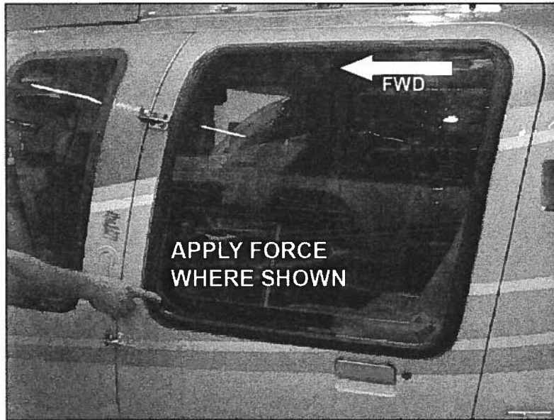
FIGURE 9 – INGRESS VERIFICATION TEST
