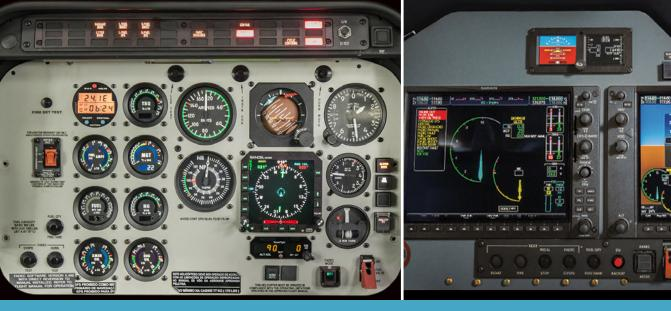
The Bell 407 G1000 NXi Retrofit Kit is designed for Bell 407 Aircraft SN 53000-54299
