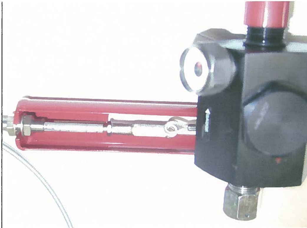
Figure 4 Cable Shroud Rigging
