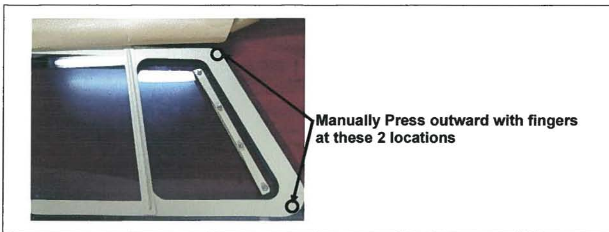
FIGURE 4 – Push Test Locations
