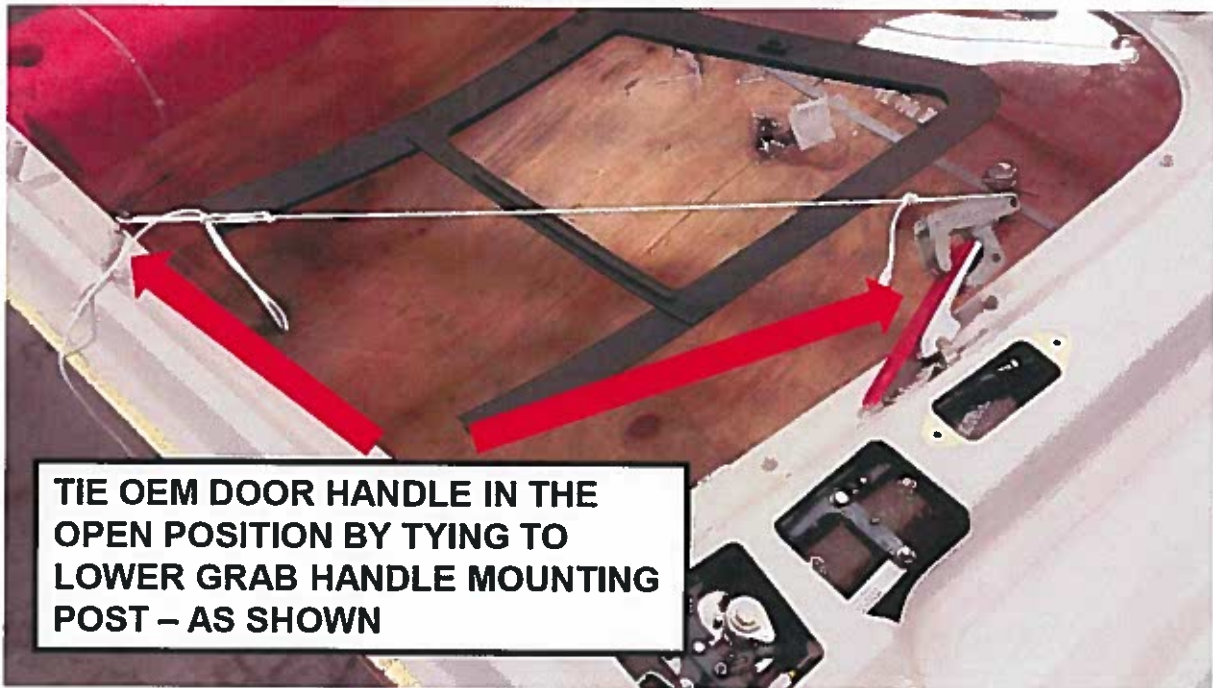
FIGURE 3 – SECURING OF HANDLES FOR RIGGING OF NEW CABLE ASSEMBLY INSTALLATION
