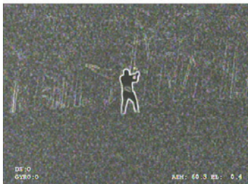
Target Outline Mode (TOM) is a high end video analytic with feature extraction that outlines the object that is different than its surroundings as it relates to IR emissivity and reflections differences in the scene.
